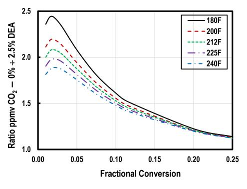
Figure 1 Effect of DEA on CO<sub>2</sub> in Gas at Equilibrium, Shown as the Ratio of ppmv CO<sub>2</sub> without DEA to ppmv CO<sub>2</sub> with 2.5 wt% DEA
