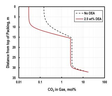
Figure 3 How CO<sub>2</sub> Concentration Changes through the Absorber (*note log scale*)
